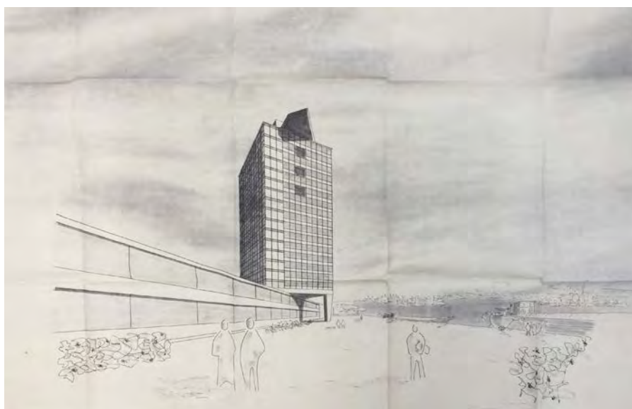
Preliminary sketch with the tower turned 45° above a low-rise volume. Image: Sandra Guarda, The Importance of Being Overhoeks .
